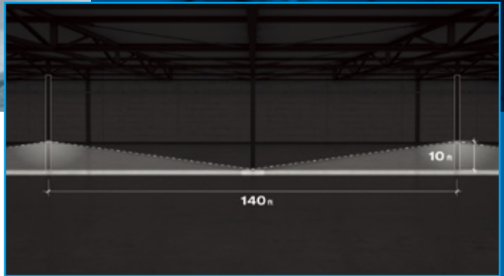
installed at 10ft in the center of the space, the spacing is at 140ft
