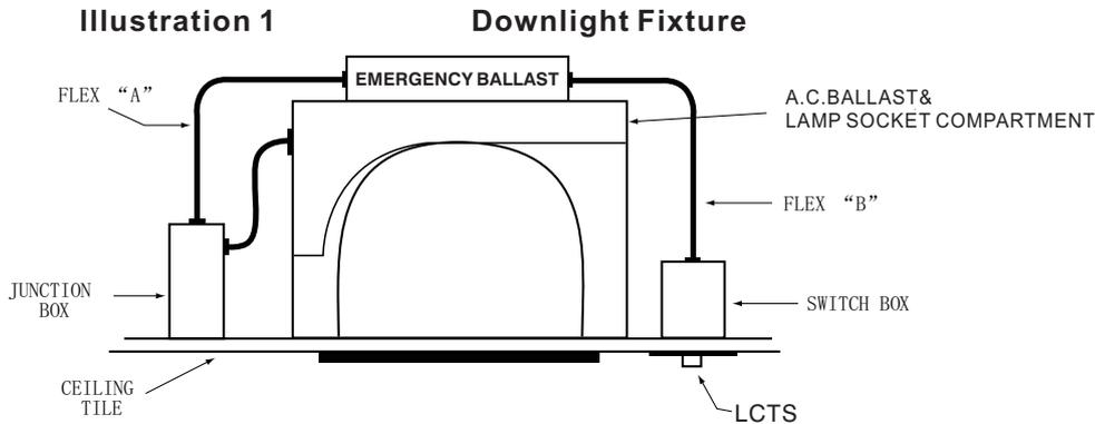
When battery packs are remote mounted, the remote distance cannot exceed  $\frac{1}{2}$  of the distance from ballast to lamp(s) specified by the A.C. ballast manufacturer. Under no circumstances should the battery pack exceed a distance 10' from the lamp.
