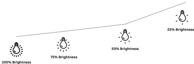
During a power outage, the emergency fixtures are dimmed to field selectable levels of 25%, 50% or 75% brightness output. Reducing wattage draw from the fixture will allow for more fixtures to be connected to the Mini Inverter, offering an extremely versatile solution for many applications.
