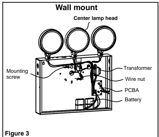
8. Our system can accept input voltages of 120 VAC or 277 VAC. Therefore, connect the black (120 VAC) or orange (277 VAC) and white (common) leads to the building utility. Connect the green ground wire to the service ground (see figure 5).
